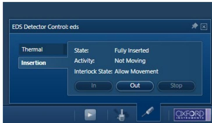
Once inserted, the State: Fully Inserted and Activity: Not Moving. In the Chamberscope view on SmartSEM:
