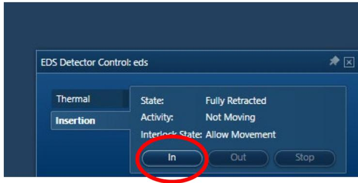
Ensure that the detector is fully retracted and not moving. Insert the detector by clicking In.
